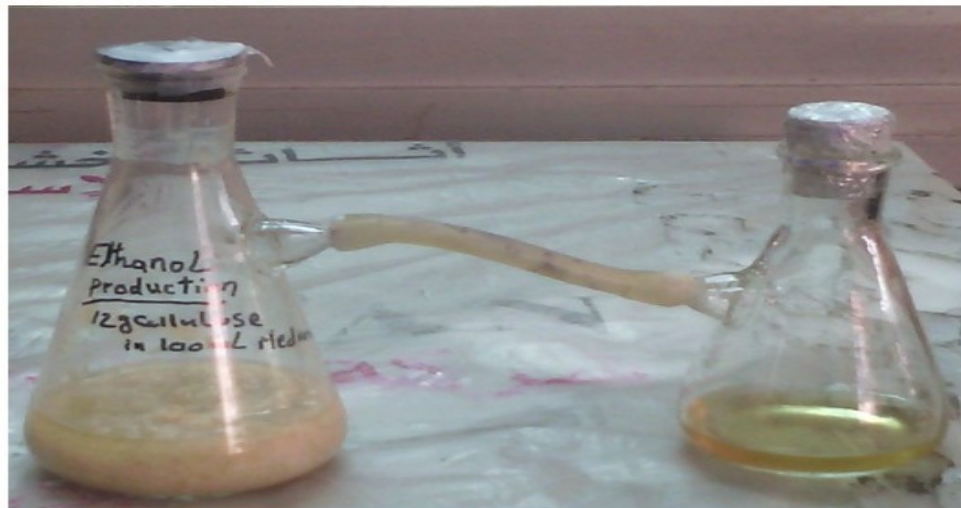
Figure.2 Simultaneous Saccharification and Fermentation of Cellulose by Saccharomyces cerevisiae and Cellulases
