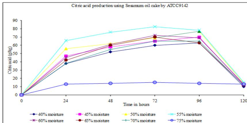
**Fig.2** Production of Citric Acid at Various Moisture Grades Using Sesamum Oil Cake as the Substrate
