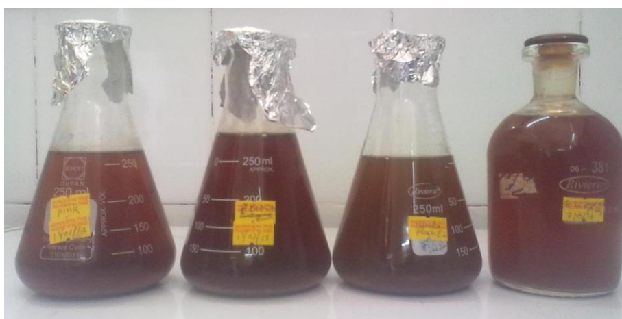
Fig.3 Black Liquor Collected after Pulping of Rice Straw
