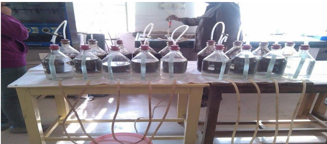
Fig.1 Experimental setup of batch model of biogas digester
