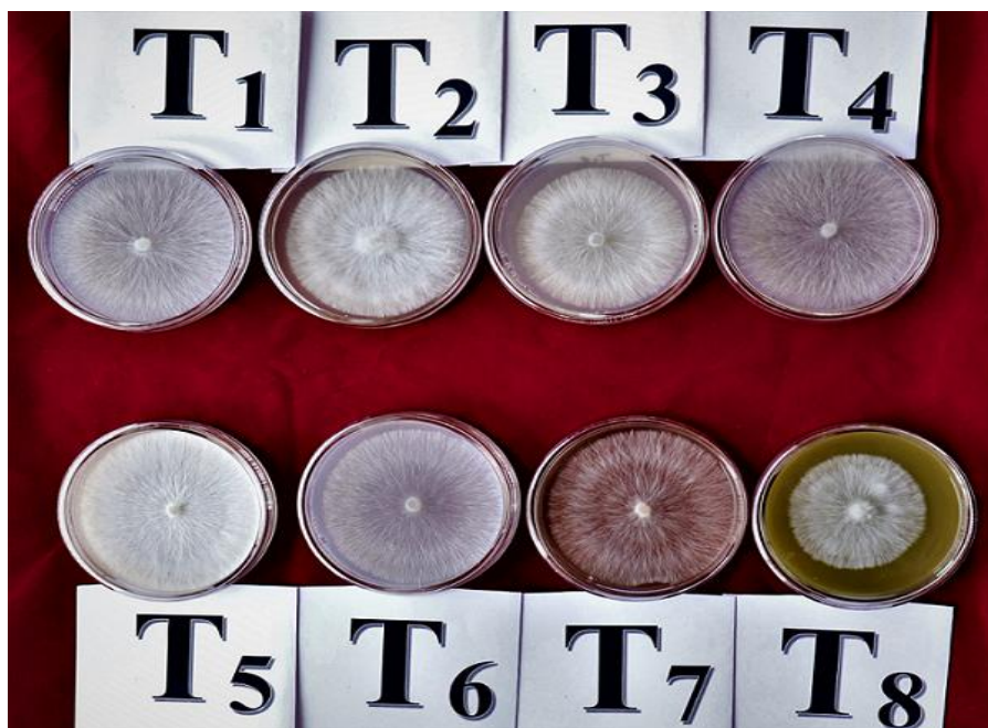
T 1 =Potato dextrose agar (Natural), T 2 =Potato dextrose agar (Hi-Media), T 3 =V-8 juice agar (Hi-Media), T 4 =C-zepak's agar (Hi-Media), T 5 =Oat meal agar (Hi-Media), T 6 =Corn meal agar, T 7 =Chickpea seed meal extract agar, T 8 =Chickpea stem extract agar Plate.1(a) Effect of different solid media on mycelial growth of S. rolfsii (96 hrs. after inoculation)
