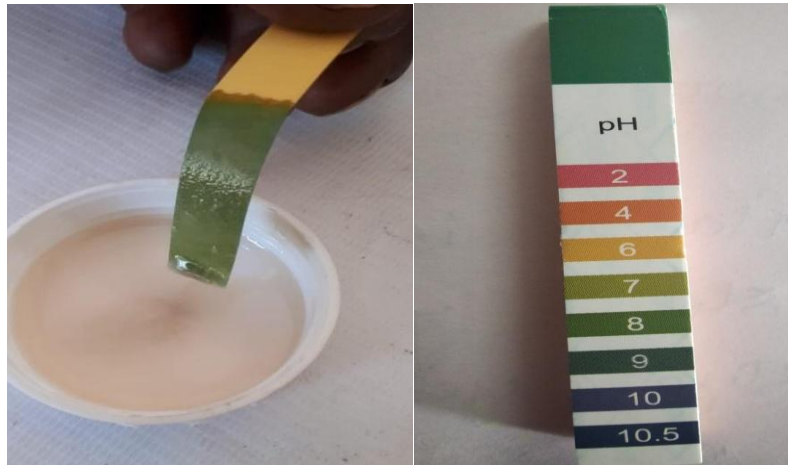
Fig.2 Identifying PH of Milk (Recorded as 7- 8, positive for mastitis)
