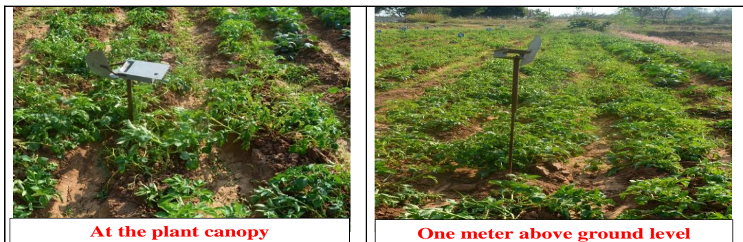
Plate.1 View of Spore trap installed in potato field at plant canopy and at one meter above ground level to quantify spore number
