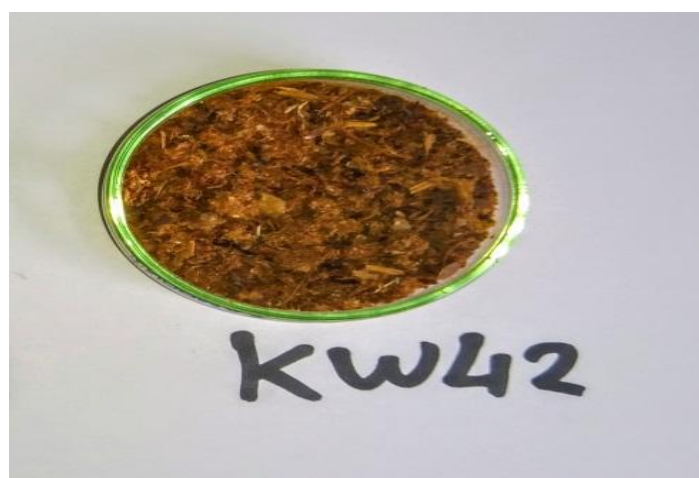
Fig.1 The dead biomass of Kw42 that was used for biosorption of Cu 2+ , Pb 2+ and Cd 2+ from wastewater
