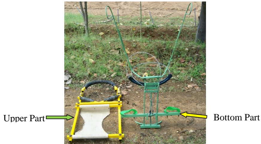
Fig.2 Upper part of modified coconut tree climber
