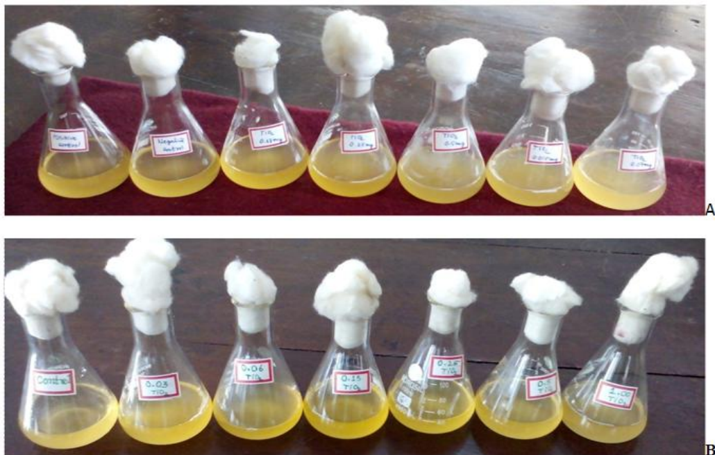
Fig.4 Effect of TiO 2 in Liquid Media of Ce-doped (A) and Un-doped (B)TiO 2 Nanoparticles
