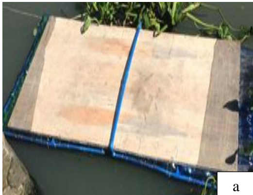
Figure.2 Another raft was tested at the Pasig River a 4.7 x 9.4 feet of fly wood with 105 pcs of plastic bottles (1.5 Lt capacity). (a) Recycled raft (b) the Prototyped design
