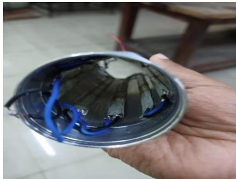
Figure.6 LED strips inside the chamber
