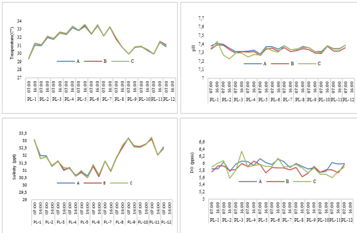
Fig.6 Water quality measurements for temperature, salinity, pH and dissolved oxygen parameters
