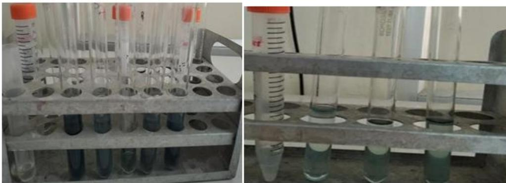
**Fig.8** Experimental setup for weight loss measurement of mild steel coupon in cooling water at various systems.
