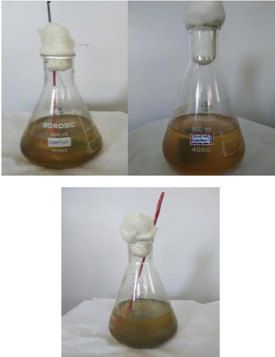
Fig.9 Photograph view of corroded mild steel surface at various weight loss experimental systems
