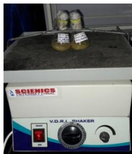
Fig.11 Control and test sample on rotary shaker at 120 rpm
